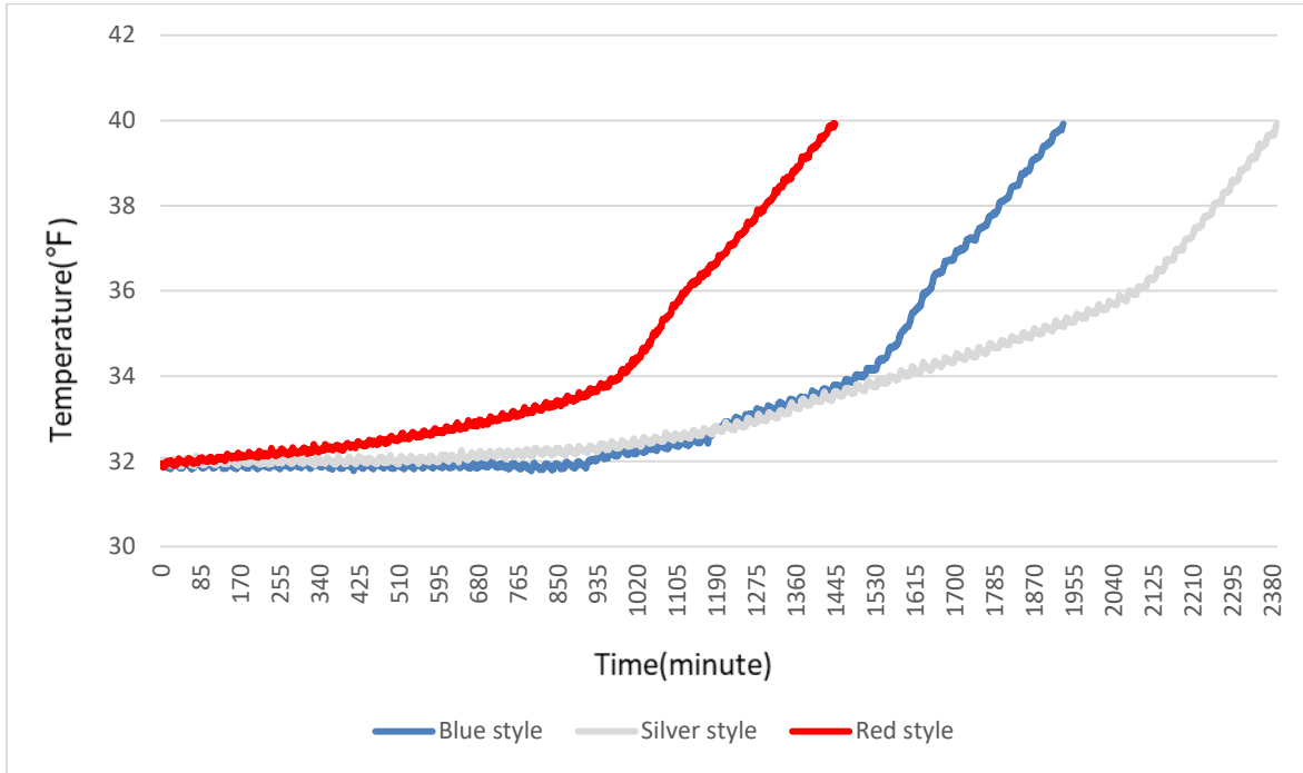
Graph 1 - Cold Retention of Copper Vacuum Insulated Bottle 17oz
